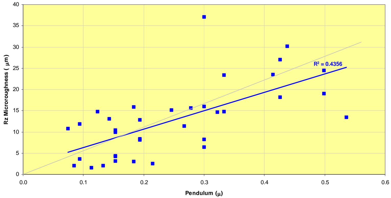
**Chart 3.5:** Pendulum CoF values and Mean Rz Surface Microroughness values.
