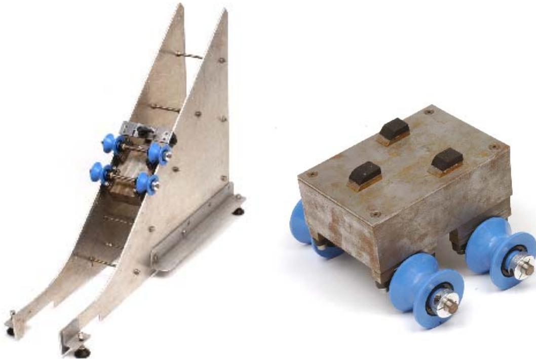
**Figure 2.3:** [a] The Kirchberg Rolling Slider, [b] Underside showing slider arrangement.
