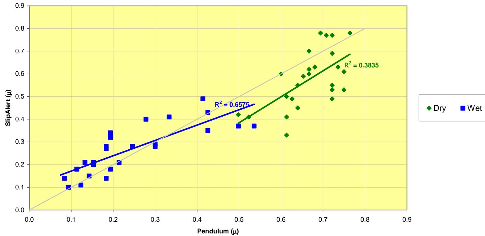
**Chart 3.4:** Pendulum CoF values and SlipAlert CoF values (calculated from median of last five of eight runs).
