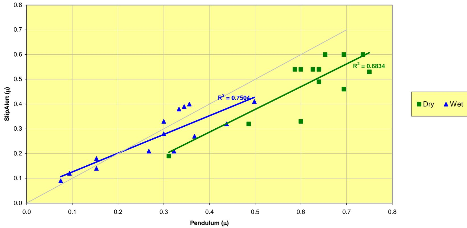
**Chart 3.3:** Pendulum CoF values and SlipAlert CoF values (calculated from mean of three runs).
